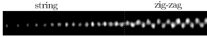
Figure 5. Fluorescence image of the left half of a stationary ion crystal with N_b \approx 68 ions in the PALLAS storage ring. The gradual transition from a string-like structure on the outside to a zig-zag inside the crystal is visible. The inter-ion spacing is comparable to that in figure 2, the trap parameter is \beta = 73 ( \omega_{\text{sec}} = 2\pi \times 180 kHz, \omega_z = 2\pi \times 21 kHz).
